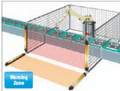
Dividing the zone between series-connected sensors
