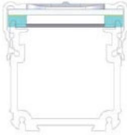
Protects the sensor from entry of the coolant that runs around the sensor.
