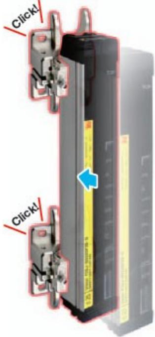
Mount the one-touch brackets to the main sensor body. Use the clamps to tightly clamp the upper body of the sensor while lightly clasping the lower body.
