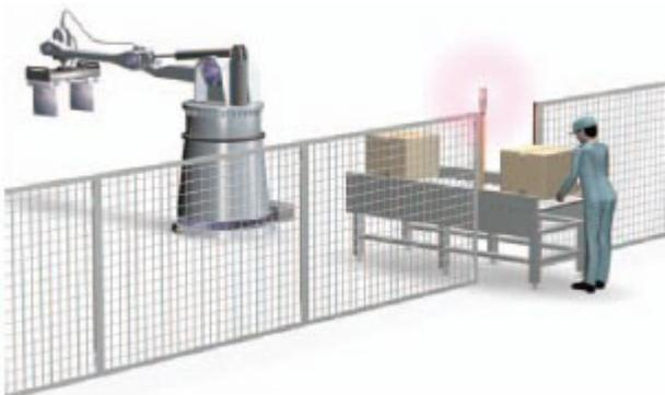
This is used in applications where the workpiece is set in position each time by an operator, and then a turntable or positioning robot moves the workpiece to the area where the work is done. A limit switch or other means is used to detect when the robot is in a safe position, and muting is then applied.
