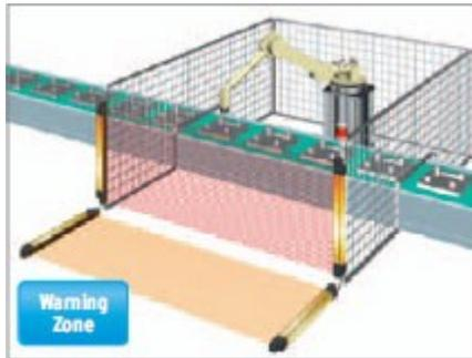
Dividing the zone between series-connected sensors
