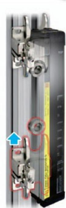
Slide the lower bracket up towards the lower circular fixture and tightly clamp the lower body of the sensor. Once done, mounting is concluded.
